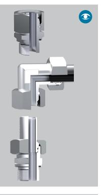
Assembly of taper coupling
